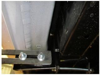
CLAMP BRACKETS TO CHASSIS (6 BRACKETS FOR DUAL CAB & 4 BRACKETS FOR SINGLE CAB & EXTRA CAB)
