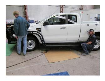
Slide Rails onto Spigots of Bar
