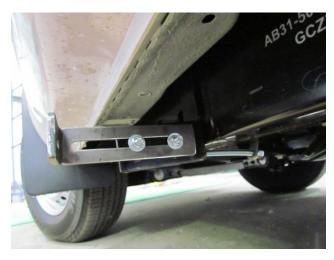
ATTACH - L SHAPED SLOTTED BRACKETS LOOSELY TO CHASSIS BRACKETS – BRACKETS POINT BACKWARDS
