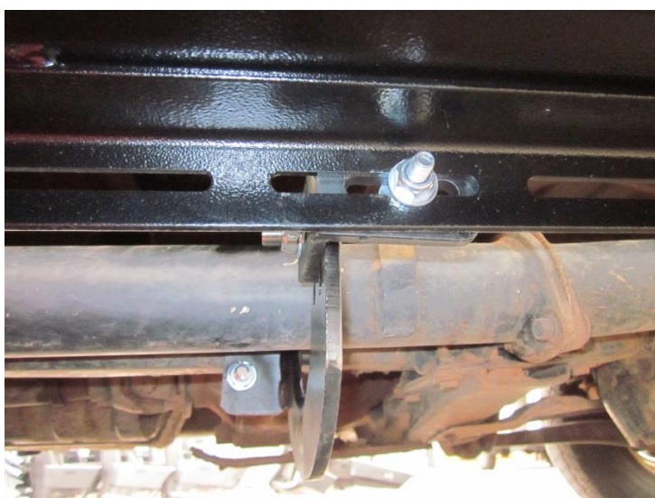
IMPORTANT – START WITH DRIVERS SIDE! Drivers side front bracket – fits around the exhaust as shown
