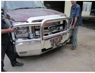
Place bullbar onto the brackets. bolt it up loosely with washers and 12 mm nuts. align the bullbar left and right and make sure that the wings follow the line of the vehicle. tighten all bolts
