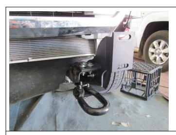
Fit bracket to end of chassis rail using the bolts provided. also ensuring the tow eyes are attached to tag provided on bracket
