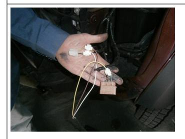
Connect the wiring kit supplied to wiring harness using wire taps & solder wiring goes under & behind headlights
