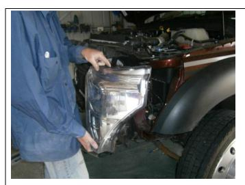
Remove head light to gain access to wiring harness to attach indicator park light leads
